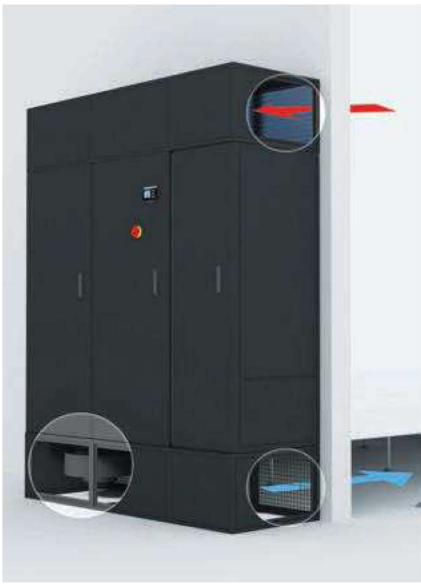
Version for installation outside the Data Centre, without raised floor, rear air supply. In this case the plinth (fixed height 550 mm) is supplied with side closure panels and rear supply air grilles. Installation of the plenum with rear re-intake system is optional, if there is no ductwork.
