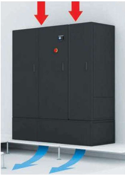
Version for perimeteral installation inside the Data Centre with raised floor height less than 550 mm. In this case, the plinth with fixed height of 550 mm is supplied with lateral closure panels and must be installed above the floor. It is essential to check that the height of the ceiling is sufficient to ensure good air suction.
