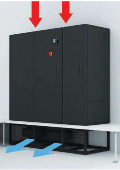
Standard version for perimeteral installation inside the Data Centre: the height of the raised floor must be minimum 550 mm.
