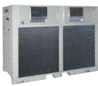
YLHD Air to water heat pump Scroll compressor / R410A Hot water up to 50°C Heating capacity: 23 to 160 kW
